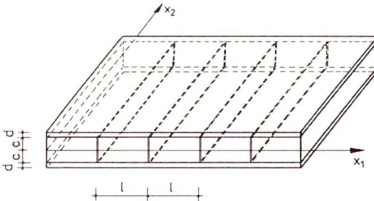
FIG. 2. Laminate with infinite aligned cracks.
