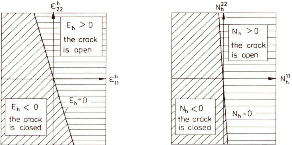
FIG. 4. a.  $(\varepsilon_{11}^h, \varepsilon_{22}^h)$ -plane; condition  $E_h > 0$  for the crack opening in the glass/epoxy  $[0^\circ, 90^\circ_3]_s$  laminate tested by HIGHSMITH and REIFSNIDER [6];  $E_h = 0.4298\varepsilon_{11}^h + 0.1286\varepsilon_{22}^h$ . b.  $(N_h^{11}, N_h^{22})$ -plane. Condition  $N_h > 0$  for the crack opening; the same laminate,  $N_h = 0.632N_h^{11} + 0.0408N_h^{22}$ .
