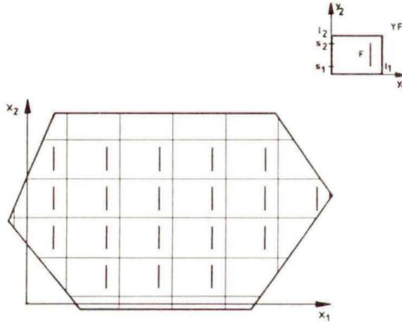
FIG. 1. Laminate with short aligned cracks.
